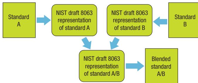
**Figure 1.** An intermediate representation for standards blending. The primitives and elements of the draft National Institute of Standards and Technology (NIST) Interagency Report 8063 can be extracted from standards A and B, reconciled into an intermediate representation, and then translated into a blended standard, A/B.
